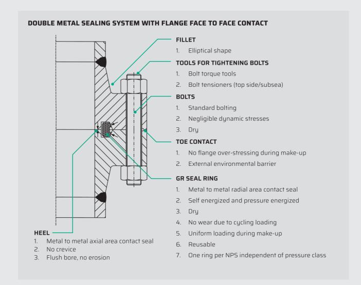
The GC-Compact® Flange uses the Galperti seal ring (GR) which seals in the flange groove. The seal ring design is based on design principles used for the wellestablished G-Lok seal ring. The heel seal ensures a smooth bore with no crevice between the flange halves at the bore. Furthermore, it reduces the area exposed by pressure to a minimum and keeps the seal ring dry during normal operations.
