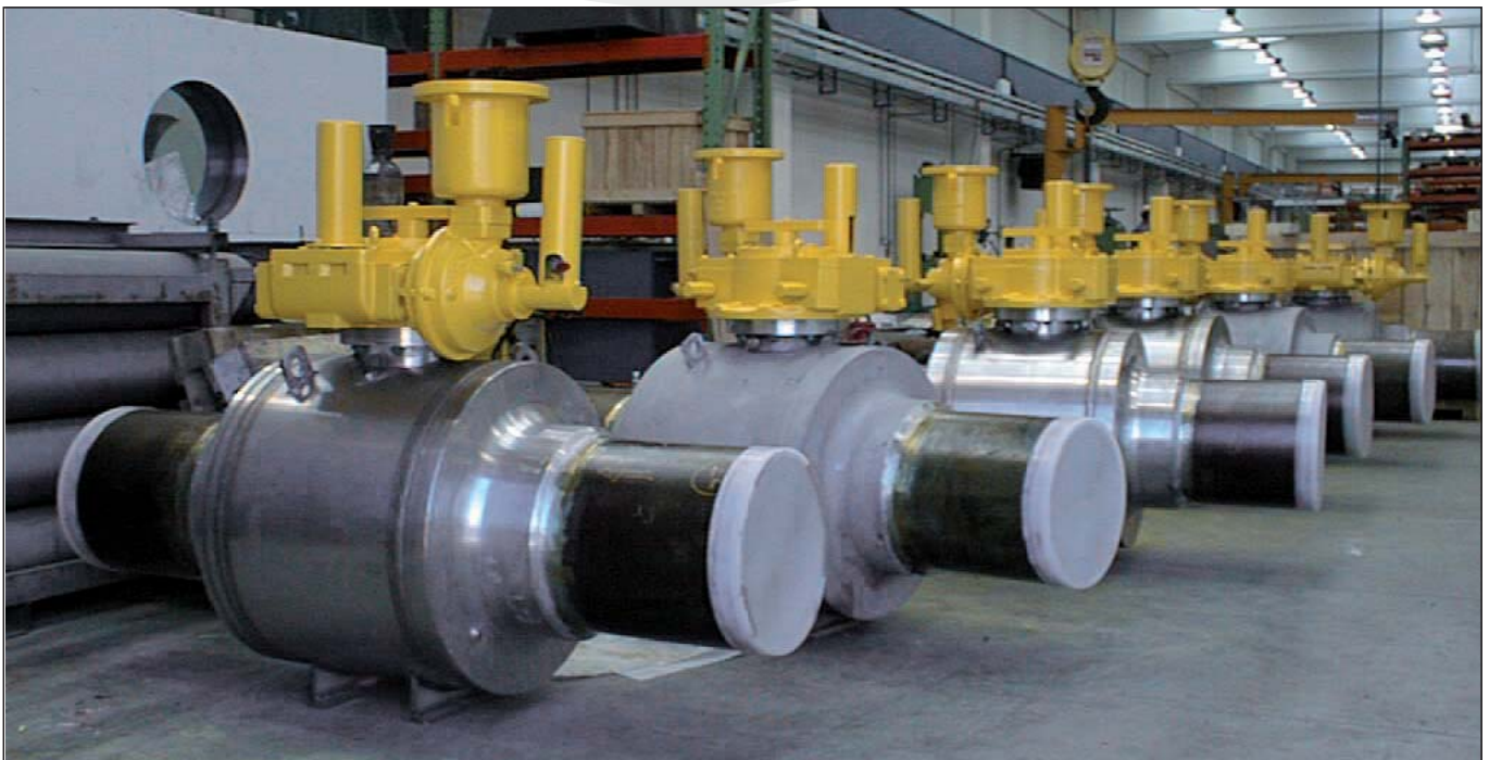
16" 600# FULLY WELDED METAL SEATED
